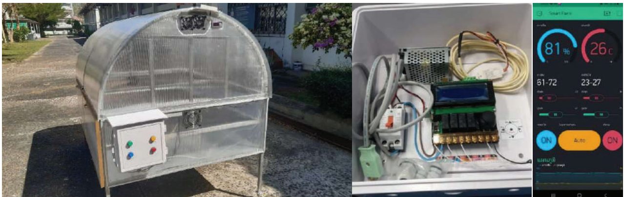
Figure 4 Install the machine and temperature and humidity control system.
