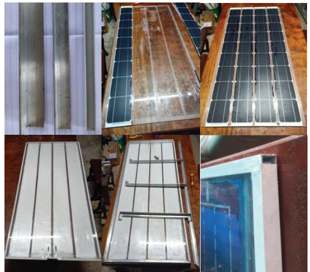
Figure 3 Construction details of the SPVT module
