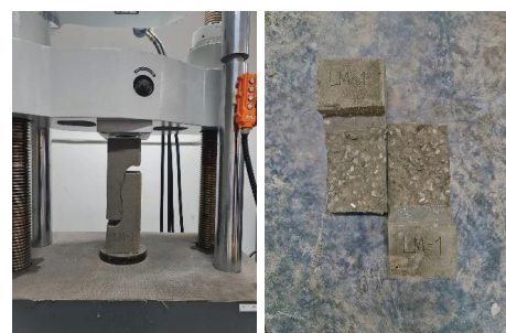
(b) LM Sample failure
