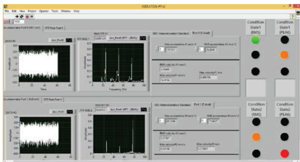
Figures 3. Vibration diagnostic systems based on Fuzzy logic Follow ISO 10816-3 Type G2/4 Rigid Speed 1500 RPM.
