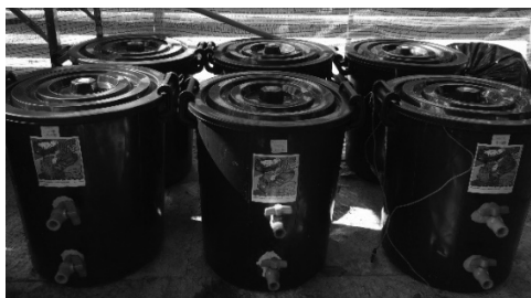
Figure 1 Single-chamber Microbial fuel cell used in this study
