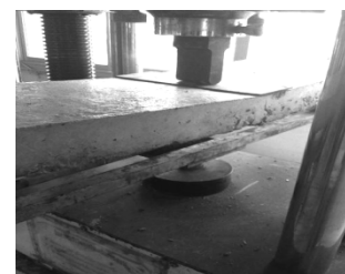
Figure 11 Test specimen bending machine
