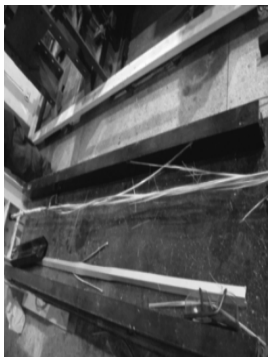
Figure 8 Sample of tensile strength test of hot rolled bamboo twisted
