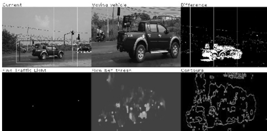
Figure 2 Screen shot after detecting a red light runner using hand held 1900 _ 1080 pixel cell phone camera (Samsung Galaxy Grand Prime)
