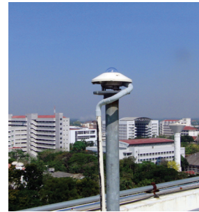
Figure 3 The pyranometer for measuring solar irradiance
