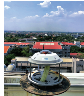
Figure 4 The sky camera for measuring cloud cover
