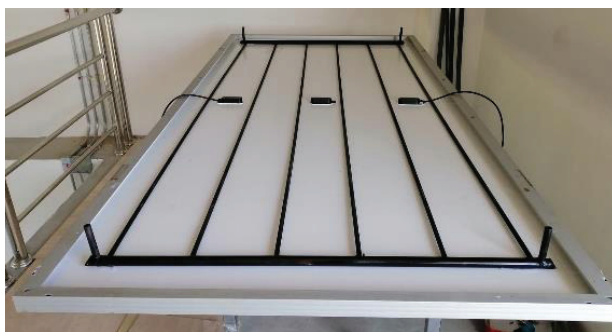
Figure 4 Heat sink under solar cell (Design)
