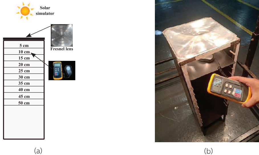
Figure 3 (a) The distance used for testing the total distance of light (focus distance), and (b) Measure the luminance of light
