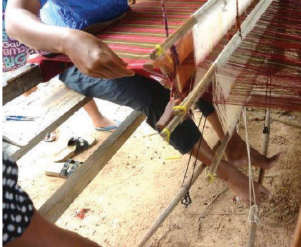
Figure 2 The use of foot pedals for wooden beams
