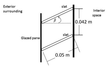
Figure 5 Side view of two adjacent slats
