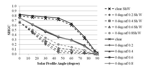
Figure 1 SHGC and ShW SHGC of the window with the blind in different slat reflectances when the slat is set at  $0^{\circ}$ . ref = slat reflectance. Clear = clear glass window.
