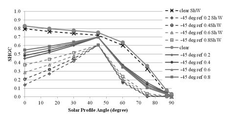
Figure 3 SHGC and ShW SHGC of the window with blind in different slat reflectances when the slat is set at -45°. ref = slat reflectance. Clear = clear glass window.
