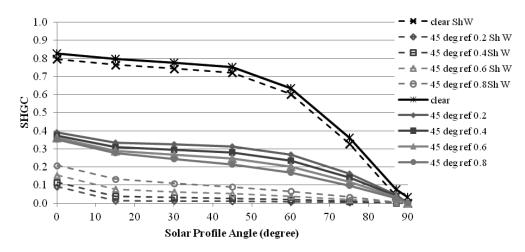
**Figure 2** SHGC and ShW SHGC of the window with blind in different slat reflectances when the slat is set at 45°. ref = slat reflectance. Clear = clear glass window.
