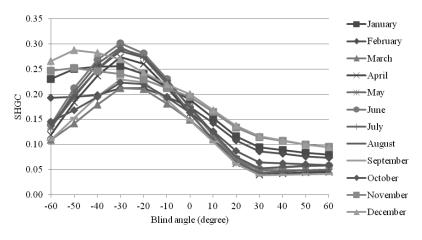
Figure 8 The monthly effective SHGC of the double-pane window with blind
