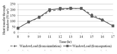
Figure 11 The heat transfer through window on the example date
