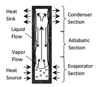
Figure 1 A schematic of the Thermosyphon<sup>10</sup>
