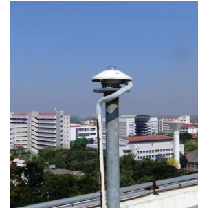
Figure 3 The pyranometer for measuring solar irradiance
