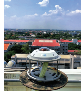
Figure 4 The sky camera for measuring cloud cover
