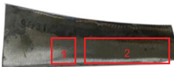
Figure 2 The big knife made of low carbon steel and positions for test pieces
