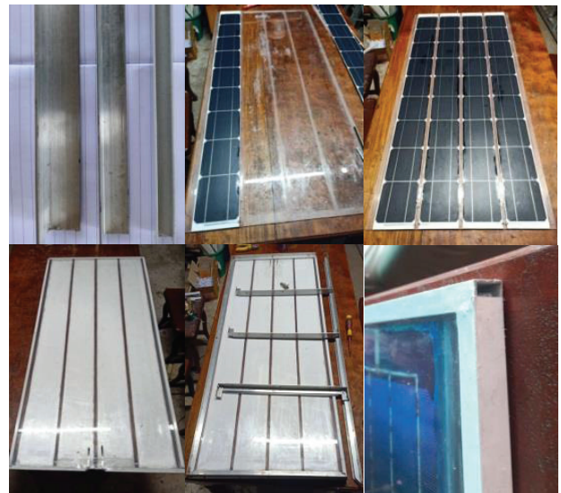
Figure 3 Construction details of the SPVT module
