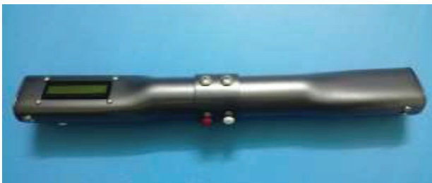
Figure 8 A prototype of a portable height measuring device
