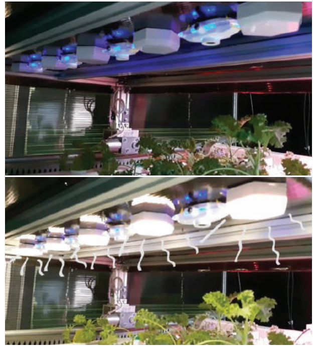
Figure 7 Camera detecting the growth of vegetables
