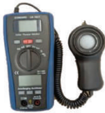
(c) Solar power meter
