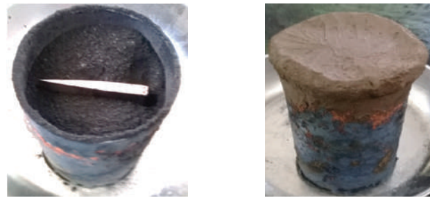
Figure 4 (a) A part of the big knife embedded in a carburizing box (b) The lid of the carburizing box was sealed using clay
