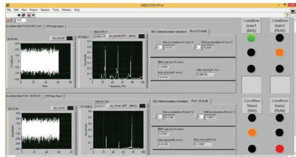
Figures 3. Vibration diagnostic systems based on Fuzzy logic Follow ISO 10816-3 Type G2/4 Rigid Speed 1500 RPM.
