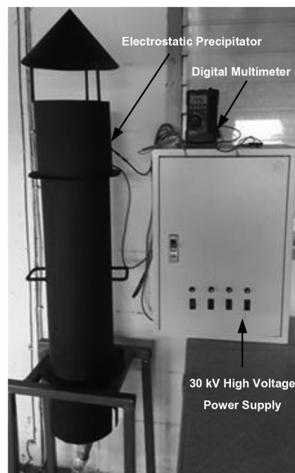
Figure 10 Prototype of the developed electrostatic collector for tobacco monopoly exhaust
