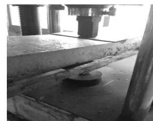
Figure 11 Test specimen bending machine
