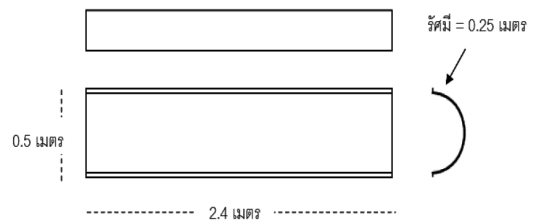
Figure 3 Size turbine blades (top view, front view, beside view)
