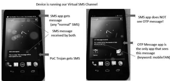
Figure 12 SMS attacking by Mobile Trojans
