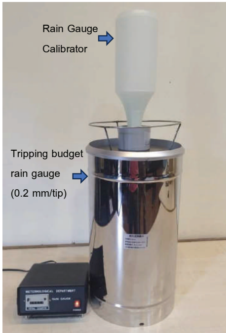
Figure 3 Tripping budget rain gauge (0.2 mm/tip) and calibration kit
