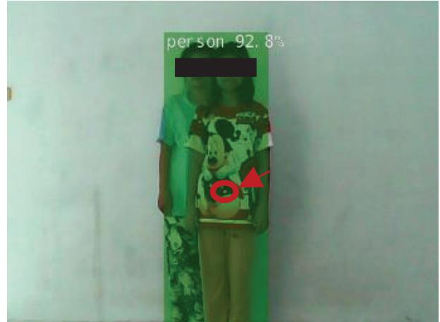
Figure 23 Detecting a person standing stacked with in an image that only one person can be detected by the system
