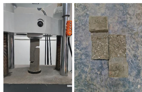
(b) LM Sample failure
