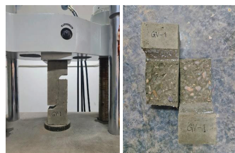
(a) GV Sample failure
