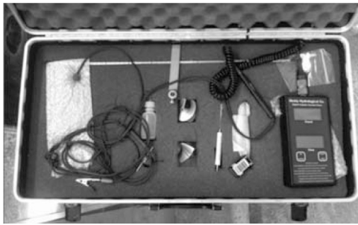
Figure 11 Miniature current meter
