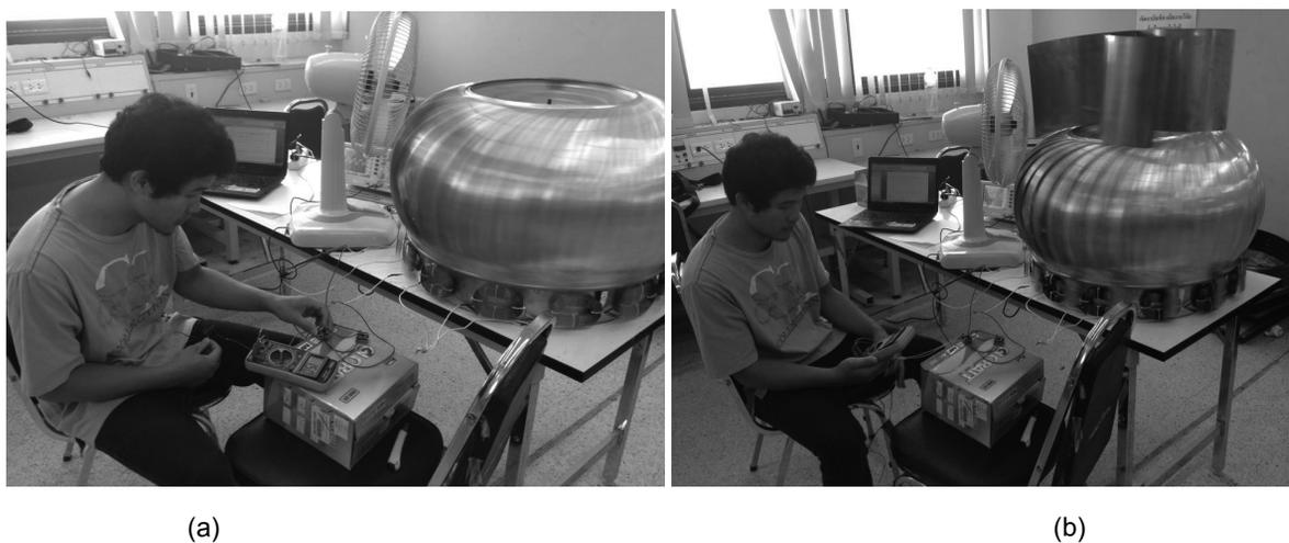
**Figure 2** Photographs of the experimental test systems: (a) testing the conventional RVWG and (b) testing the proposed RVWG
